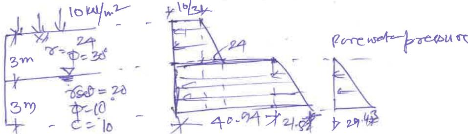
$$K_{a1} = \frac{1}{3}, \quad \sigma_h = \frac{1}{3} \times 10 + \frac{1}{3} \times 24 \times z, \quad \text{when } z = 0, \quad \sigma_h = \frac{10}{3} \\ z = 3\text{m}, \quad \sigma_h = \frac{10}{3} + 24 =$$
