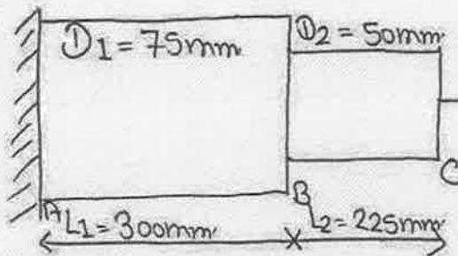
$$E = 6 \text{ GPa} \\ = 6 \times 10^3 \text{ N/mm}^2 \\ K = 50 \text{ MN/m.} = 50 \text{ kN/mm}$$
