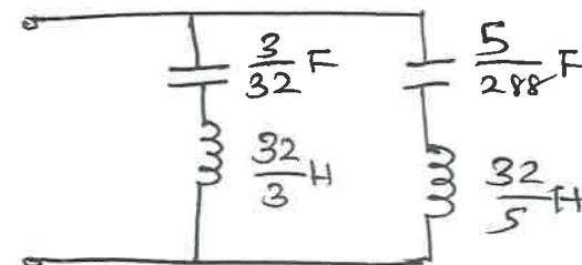
II Cauer I realization1) Continued fraction expansion of  $Z(s)$  (2marks)2) finding the component values and drawing
