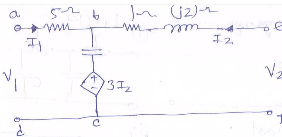
Applying KVL to loop abcd in above fig.
