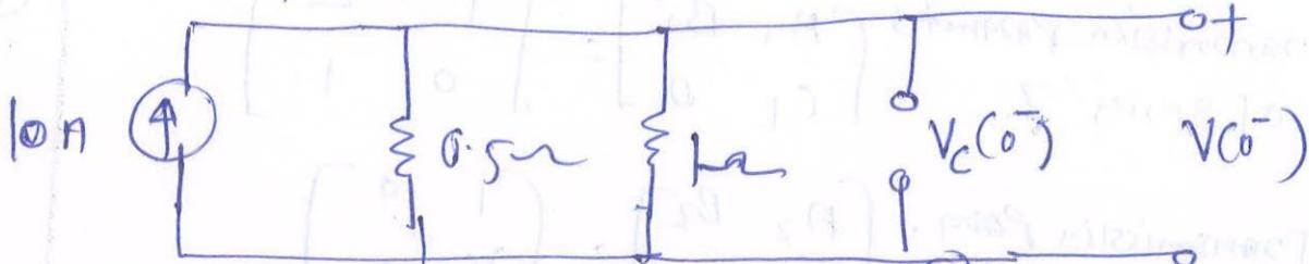
At  $t=0^-$ , the network attains Steady state condition
