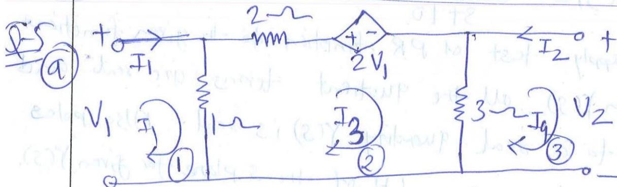
$$\text{For loop } ① \quad I_1 - I_3 = V_1 \quad ①$$
