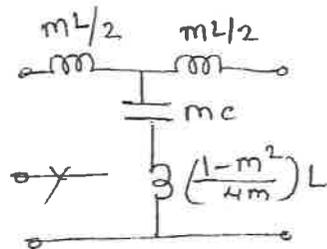
$$\frac{mL}{2} = 0.2264 \times 3.978 \mu\text{H} = 0.9006 \mu\text{H}$$
