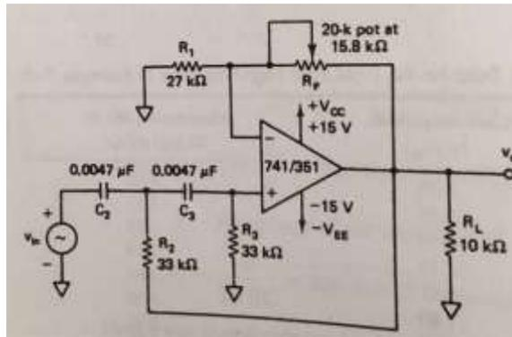
$$f_L = \frac{1}{2\pi\sqrt{R_2 R_3 C_2 C_3}}$$
