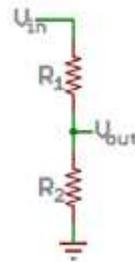
At  $20^\circ\text{C}$ , the thermistor resistor will be  $3.5\text{K}\Omega$ , and the divider voltage will be
