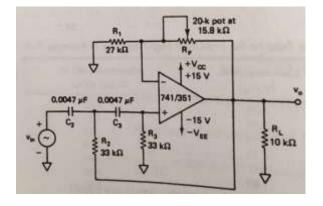
$$f_L = \frac{1}{2\pi\sqrt{R_2R_3C_2C_3}}$$
