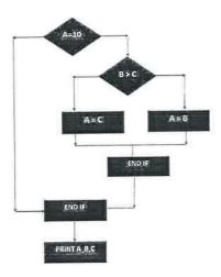
The Cyclomatic complexity is calculated using the above control flow diagram that shows seven nodes(shapes) and eight edges (lines), hence the cyclomatic complexity is 8 - 7 + 2 = 3
